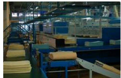
Automated linen transfer from Classic Folders (large pieces), Napkin Bottom-Up (small pieces) and the blanket folder to the Dispatch area .
