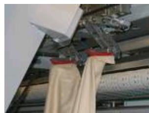
Step 3: The «Soft-Touch» spreading clamps pivot to a horizontal position.
