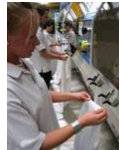
Step 1: Two corners are clipped into the height-adjustable feeding clamps.
