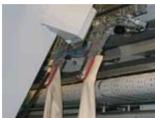
Step 2: Transfer from feeding clamps to the «Soft-Touch» spreading clamps.
