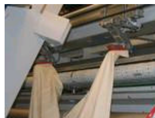
Step 4: Fast, yet gently spreading of the linen onto the vacuum beam.
