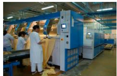
A complete ironer line: Logic 2000 feeder – Jenroll EXP ironer – Classic Folder with stacker.
